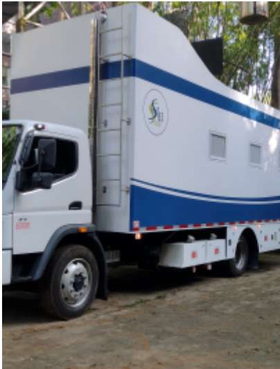
The completed unit ready for service: NINOX coachwork on a Mitsubishi Fuso F1 chassis, carrying the SIES Salud identity in a tropical Colombian setting.
