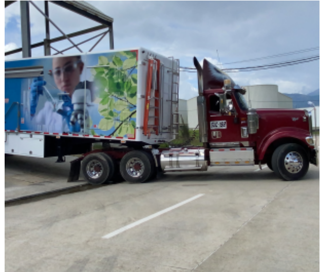
Full lateral view of the unit showing the complete truck-semitrailer assembly. The 15-meter overall length accommodates all functional laboratory zones without compromising mobility on secondary roads.
